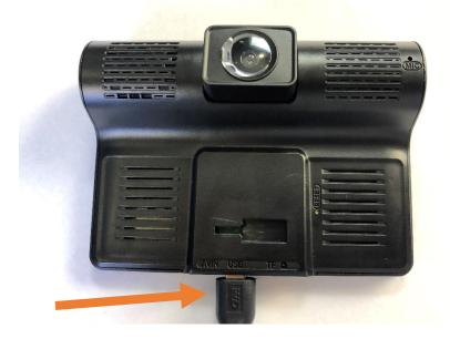
5. Turn the camera on by depressing the power button in the center on the side of the camera
