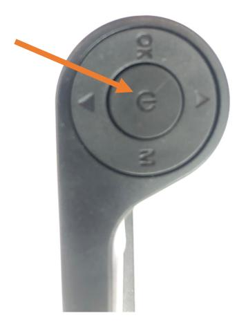
6. Press the "M" key once, and you will see the video menu (note, if the device automatically turned on and entered recording mode (flashing red light), Press the "OK" button to stop recording. Then press the "M" key and continue with these instructions.
